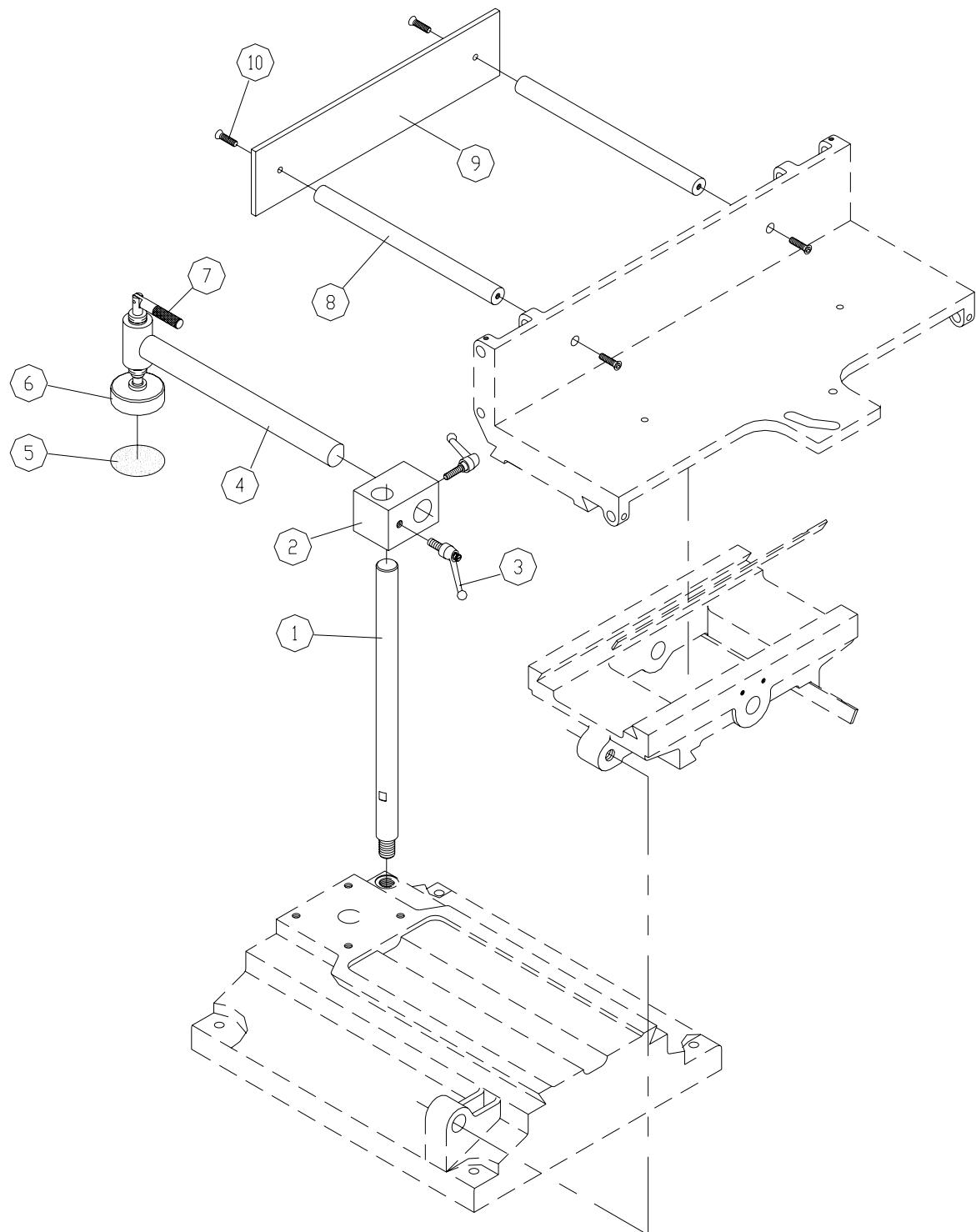
**Parts List : 719A Workpiece Hold Down Assembly (Optional)**
